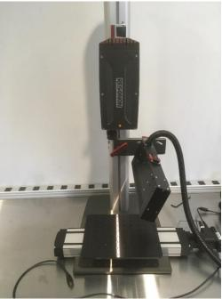
Insert the imager USB cable (or ethernet) through the cable guides at the top and bottom of the tower. Connect the cable to the camera. The imager cable (s) will be included in the packaging with your imager. XC2 shown, other imagers will be similar. Some imagers, like the NIR will use an ethernet cable and a power supply.
