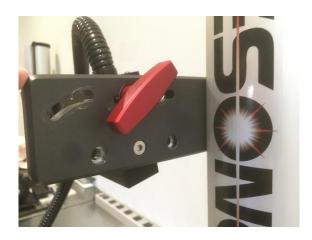
Connect the limit switch cable on the stage motor as shown.
