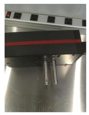
Loosen the thumbscrew on the imager mount and install the imager as shown. Tighten the thumbscrew.
