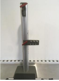
Using the 5/32" Hex Key, install the shoulder screw into the lower hole on the Light Mount as shown. Begin by using the center hole as a starting point. This can be swapped to one of the other two positions if preferred.
