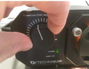
The knob on top of the line light can be used to focus the beam. The T-Handle on the back of the light mount can be used to angle the beam and the T-Handle on the front of the mount can be used to adjust the light up and down. Make sure you always have a good grasp of the line light when making adjustments with the T-Handles.
