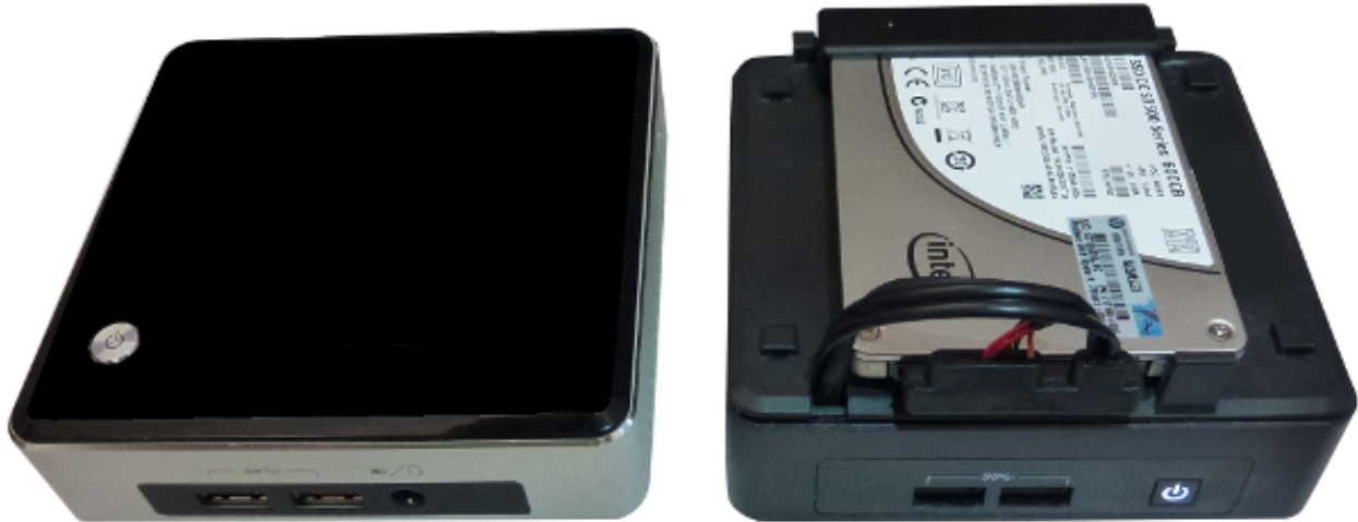
Fig. 5.4: Older Flight Computers - NUC Generations 1, 2
