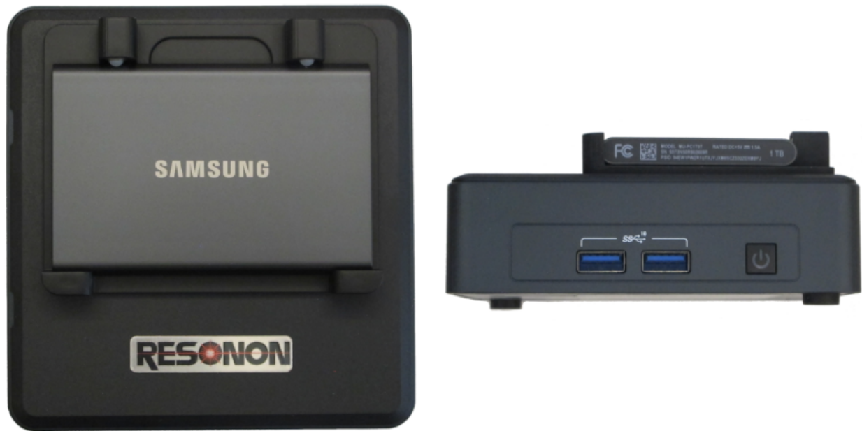
Fig. 5.2: Current Flight Computer - NUC Generation 4 top, front
