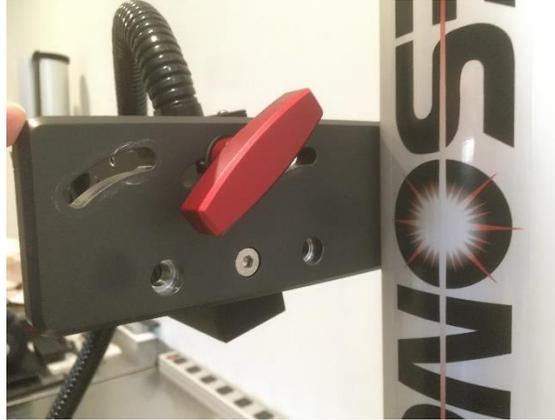
Connect the limit switch cable on the stage motor as shown.
