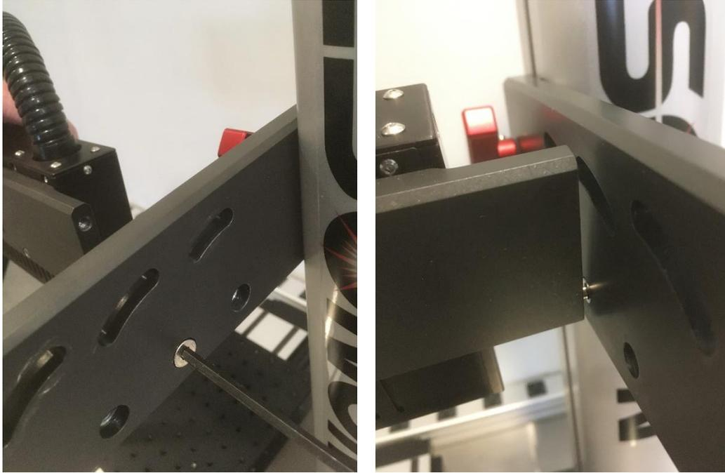
Using the T-Handle with the plastic washer installed, attach it to the top hole of the light bar through the middle slot of the Light Mount as shown. The T-Handle can be used to adjust the angle of the Line Light beam.
