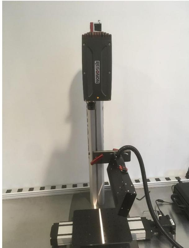
Using the T-Handle on the imager mount, you can adjust the height of the imager. Always keep a firm grasp of the imager when making height adjustments.
