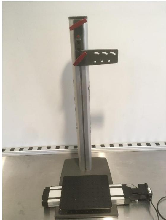
**Step 3.** Adjust the position of the Light Mount and attach the Line Light.
